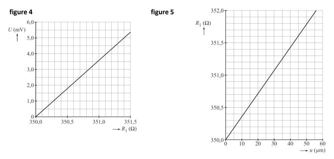
The strain gauge has a length of 6.1 cm and has been glued to a bridge cable of 198 m in length. The diagram of figure 5 shows the relationship between the resistance and the stretching of the strain gauge. If the cable of the bridge stretches 12 cm due to too much traffic, an alarm sounds.
