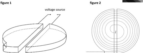
An electric field is located in the space between the two drums. Because the drums are connected to an alternating voltage source, this field keeps changing direction.
