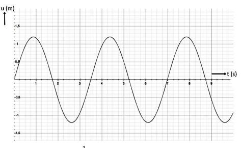
The frequency of this oscillation is given by  $f = \frac{1}{2\pi} \sqrt{g/l}$  in which *l* represents the distance of the anchor point to the centre of gravity of the gondola and *g* represents the gravitational acceleration.
